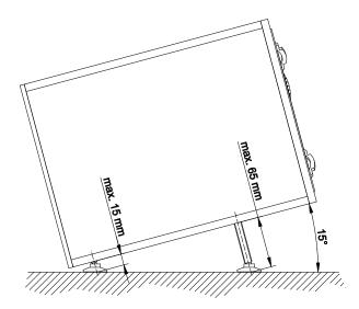
Do not operate the center speaker without the preassembled height-adjustable feet, otherwise air escapes through the threaded holes, affecting the reproduction quality.
